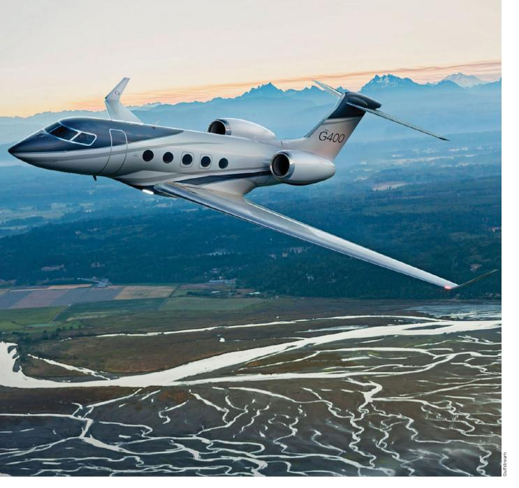
PW812GA engines – certificated by Transport Canada in mid-September – each developing almost 13,500lb (60kN) of thrust. The new model will hit its maximum 4,200nm range when cruising at Mach 0.85. Maximum cruise speed will be M0.88.
