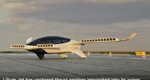
Lilium Jet has vectored thrust engines integrated into its wings
