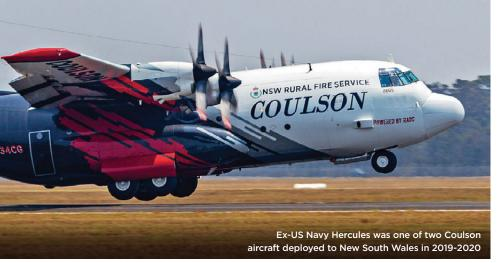
907kg pallet of firefighting gel. Including fuel, this resulted in a takeoff weight of about 66,818kg.
