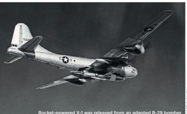
Rocket-powered X-1 was released from an adapted B-29 bomber
