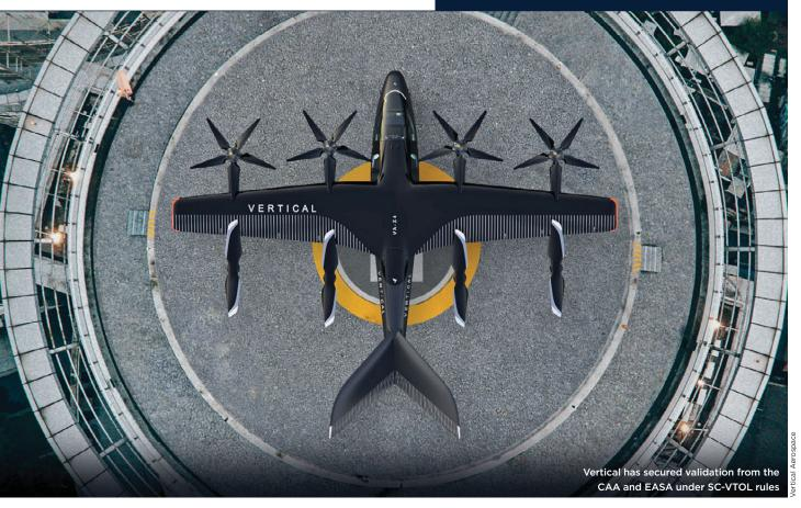
hovers, followed by thrust-borne and then wingborne flying with full transition from vertical flight to cruise. Vertical has already secured concurrent validation from both the UK Civil Aviation Authority and the European Union Aviation Safety Agency (EASA) for certification under SC-VTOL (special condition for vertical take-off and landing aircraft) rules. It hopes to follow that rapidly with approvals in key markets Brazil, Japan and the USA.
